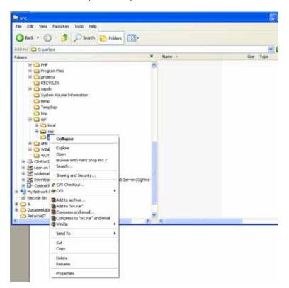
Navigate to a directory you wish to contain the source code structure, right click on the directory and select the 'CVS Checkout...' command.
